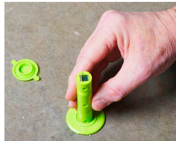
RH testing, approved by ASTM F2170, is the most accurate way to ensure that a concrete slab meets relative humidity specs for a damage-free installation
